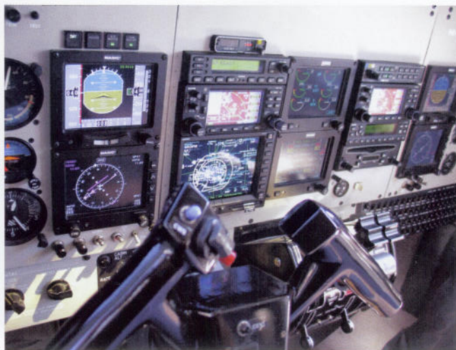
One of the Commanders has the full Meggitt panel including dual EFIS, electronic engine display, and autopilot.
