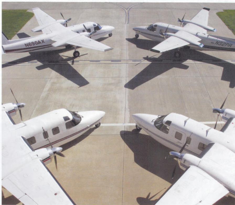
The four-Commander fleet began with an 840. The company later added two 690As and a 690B. All have TPE331-10T power. Airframe, engine, and instruments/avionics commonality was a company objective.
